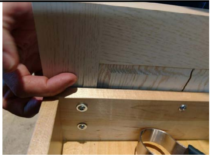
Cabinet drawer false front splitting
